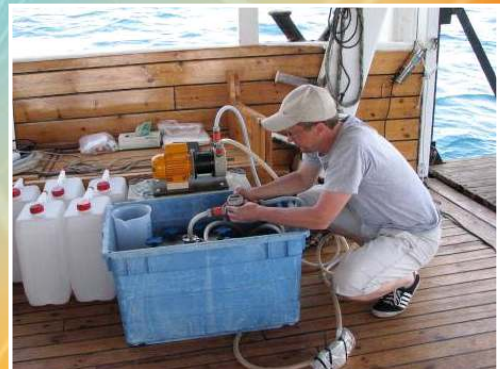
Filtration of water samples to separate particulate and dissolved fractions
