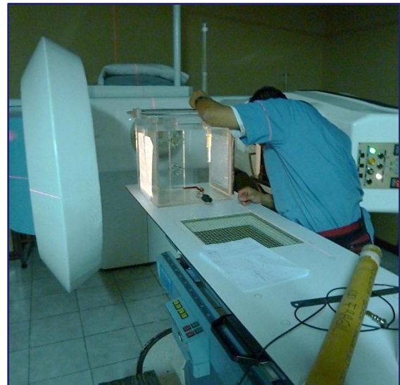
A teletherapy machine in the process of being calibrated.
