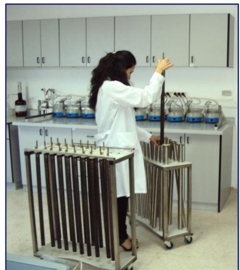
Preparation of samples for the electrolysis tritium enrichment system (LAEC).
