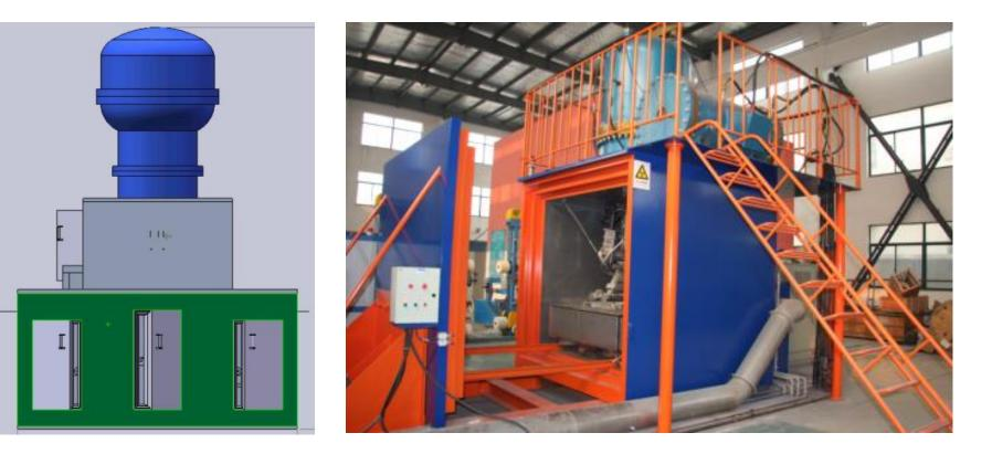
Self-shielded low energy electron accelerator
