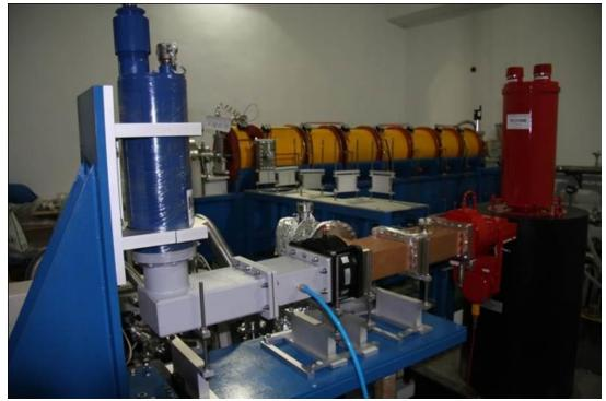
10MeV-20Kw S-band Linac electron accelerator 10MeV-40Kw L-band Linac electron accelerator
