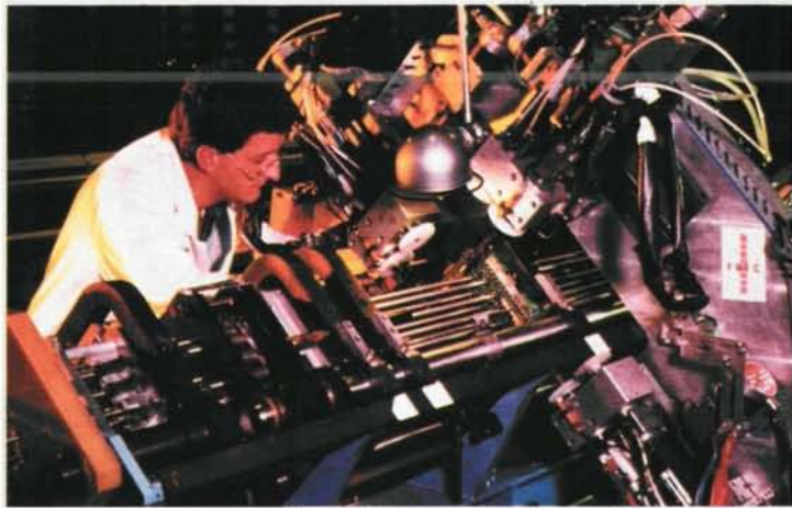
A technician inspects the structure of a fuel assembly. The integrity of fuel assemblies under various conditions can be modelled using sophisticated computer codes. Credit: Framatome.
