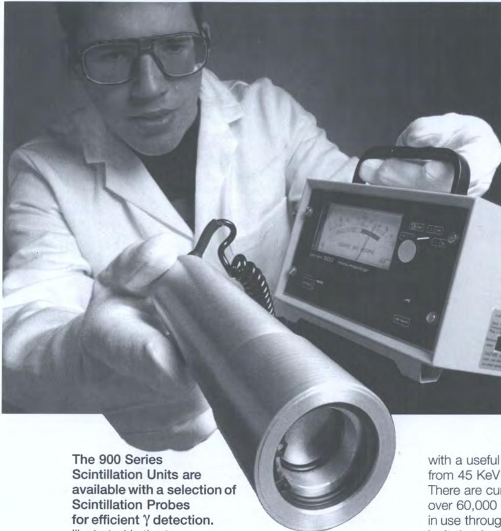
**The 900 Series Scintillation Units are available with a selection of Scintillation Probes for efficient  $\gamma$  detection.**
