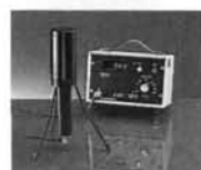
Gamma Counter using a Well Crystal Scintillation probe.
