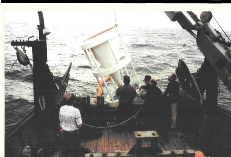
Marine research: deploying a sediment trap
