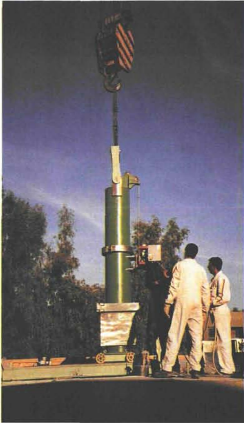
Scenes from the removal operation: Over a period of 5 months in late 1993 and early 1994, the IAEA organized and supervised the removal of all declared stocks of nuclear-weapons-grade material from Iraq's Tuwaitha Nuclear Research Centre and a nearby storage site. All told, highly enriched uranium in the form of 208 assemblies of spent nuclear fuel were recovered, cleaned, loaded into 23-ton transport casks, sealed, and flown out of Iraq. Shown here are scenes from the complex and technically demanding operation, which involved 170 workers, including Iraqi personnel, IAEA experts, and US and Russian contractors. (Credits: R. Ouvrard, IAEA; Iraq Atomic Energy Commission)
