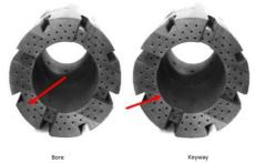
Figure 3 – Arrangement of graphite fuel bricks in AGR core
