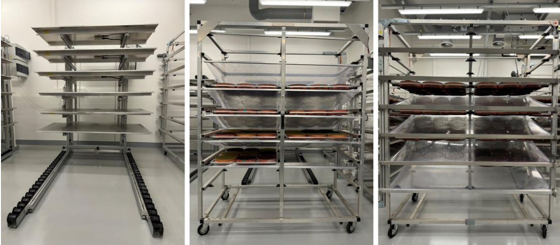
Figure 9: TPU 4 system (left feeding unit, middle holding trolley front view, and right holding trolley front back view) in the fly rearing facility of the Insect Pest Control laboratory (IPCL/ IAEA), Seibersdorf: (Source: Chantel de Beer, IPCL).
