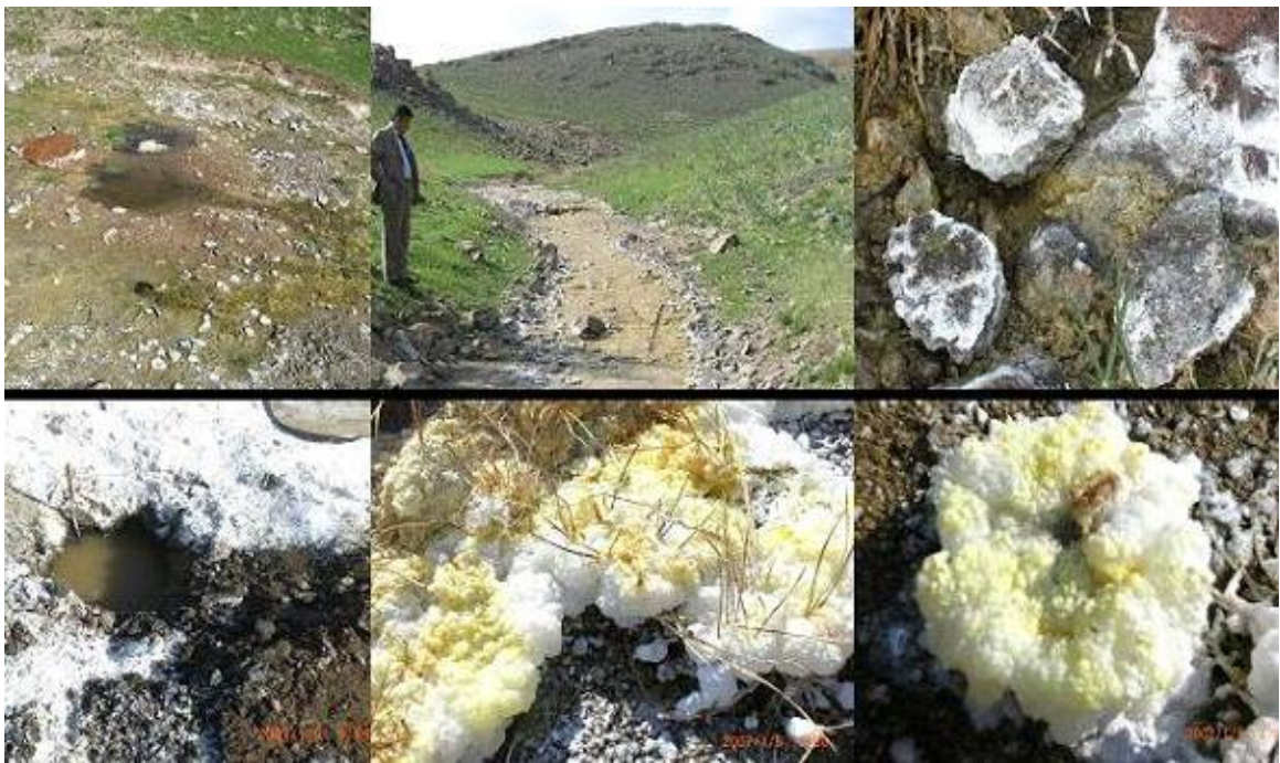
Drainage water salt deposits (with high contents of uranium in the sodium and sulphates crystals) on the bottom of the creek near the tailing dumps of I-II
