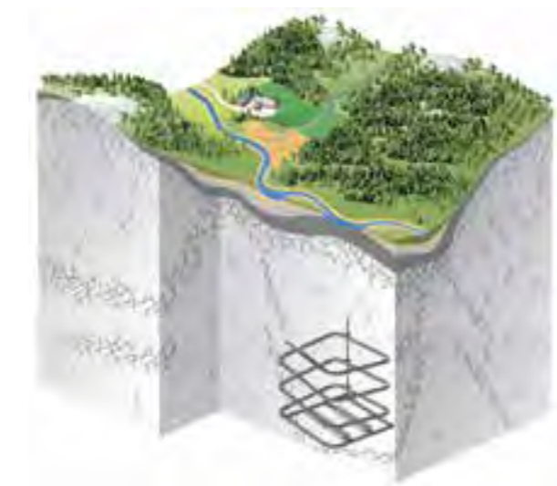
Figure A12 Illustration of the current concept for SFL as a geological repository with two different sections. Metallic waste from the nuclear power plants is placed in a waste vault (BHK) designed with a concrete barrier, and legacy waste is placed in a waste vault (BHA) designed with a bentonite barrier. An evaluation of the post-closure safety for this design was presented in 2019.
