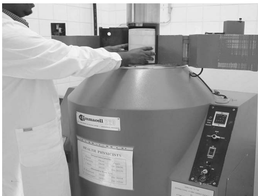
Figure 1. In preparation for irradiation, a canister of insects is placed in the irradiation chamber (while it is in the shielded position) of a self-contained gamma irradiator. Depending on the dose rate of the day, the timer on the control panel (lower right) is set to give the desired dose.
