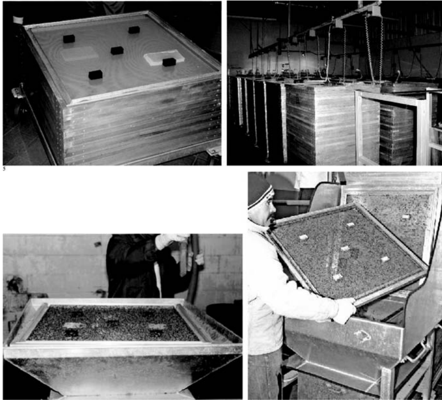
Figure 3. Stages in the emergence and collection of fruit flies using the tower system. Upper left: Screen tray with aluminium frame, showing slab of food, and red-dyed pupae in a channel around the edge; Upper right: Stacks of trays in towers, each with a fan drawing air upwards. Tower system for Mediterranean fruit fly, USDA/APHIS, Sarasota, FL, USA. (Photo from C. Caceres, reproduced with permission.) Lower left: Screen tray in cold room with emerged flies on screen, and puparia removed from channel by suction; Lower right: Chilled flies being collected in a hopper. Tower system for Mexican fruit fly, USDA/APHIS, Mission, TX, USA. (Photo from J. Worley, reproduced with permission.)
