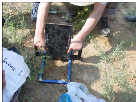
Fig.2. Soil sampling for FRN-based erosion study (Courtesy: Y. Li)
