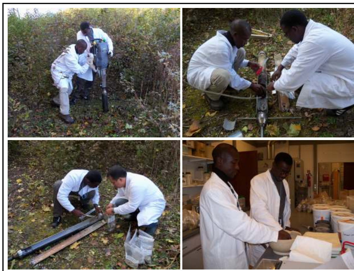
Figure 40 Soil samples collection and samples pretreatment performed by Instrumentation Unit (IU) fellows and SSU staff member in the frame of an IU and SSU collaborative training
