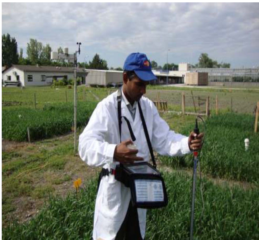
Figure 14 (b). A fellow monitoring soil water in the field using the Diviner
