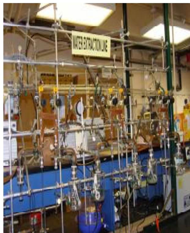
Figure 39 A cryodistillation water extraction line at the Stable Isotope Facility Laboratory, University of Wyoming, WY, USA
