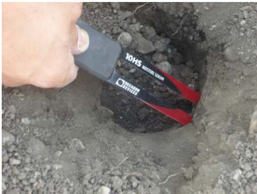
Photo 22. The new soil moisture device 10HS being installed on the field
