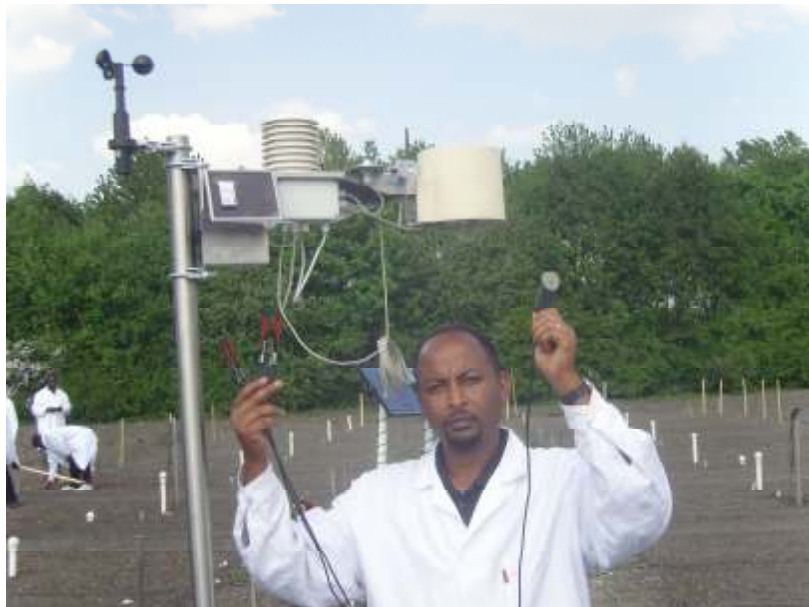
Photo 21. The imetos weather station and Decagon soil moisture sensors to be installed in the field in the field at the Agency's Laboratory, Seibersdorf
