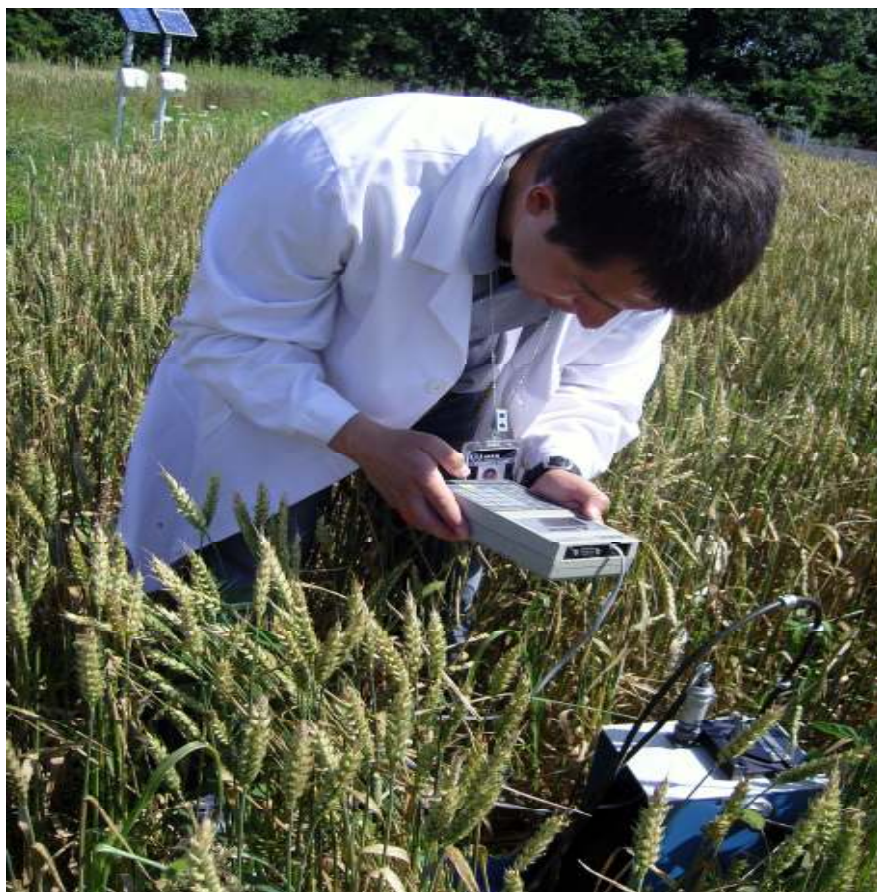
Figure 14 (a). Monitoring soil water in the field using a soil moisture neutron probe
