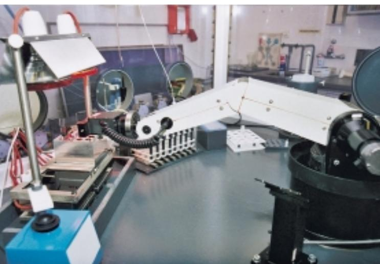
*Zymark Robot for separation of U, Pu and fission products in spent fuel samples.*
