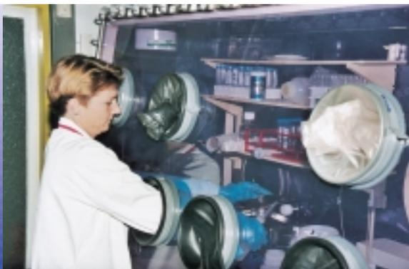
*Nuclear material samples are handled in the glove box of the ICP/MS.*
