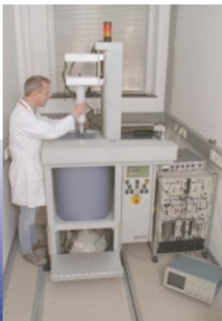
*The mass spectrometry laboratory is equipped with three mass spectrometers, including this Finnigan MAT 262 RPQ<sup>+</sup> which is used for measuring plutonium samples.*
