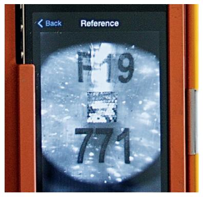
In-field verification of a fibre-optic seal by checking its unique light pattern.
