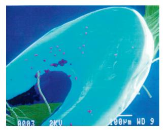
*Example of environmental sample analysis: isolation and measurement of micron-sized particles of nuclear materials to determine their isotopic composition.*
