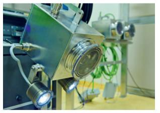
*Under water surveillance cameras installed at IAEA laboratories for testing prior to installation in nuclear ponds.*
