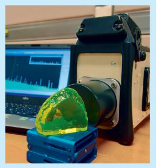
Mobile, high-resolution gamma detector for accurate measurement of the types and isotopic composition of nuclear material.
