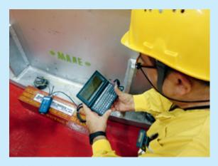
In-field verification of an electronic seal.
