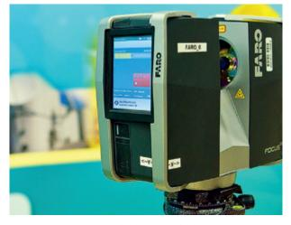
3D laser scanning allows for detection of design changes within a nuclear facility.
