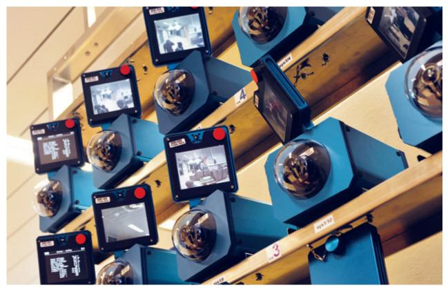
Next Generation Surveillance System (NGSS) Cameras installed at the Department of Safeguards' laboratories for testing prior to installation in nuclear facilities.
