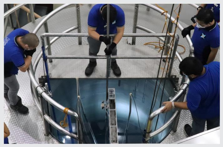
A fuel rod is loaded into the core of a subcritical assembly. (Photo: PNRI)
