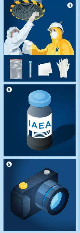
**O** Environmental swipe sample kits may be used to take samples of dust that can reveal the presence of nuclear material particles. If found, these particles can indicate if any undeclared nuclear activities have taken place (see page 10).
