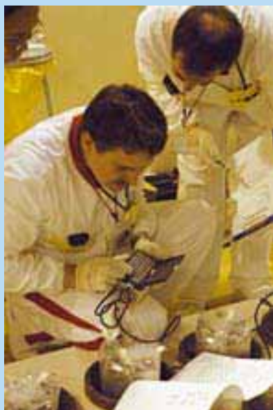
IAEA safeguards inspectors using specialised equipment, MMCA or Mini Multi-Channel Analyser, to verify fresh fuel at a nuclear power plant.
