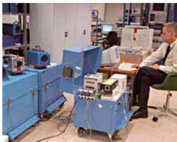
An IAEA engineer performs final testing on a remote monitoring server (Server based Digital Image Surveillance, SDIS) prior to installation in a nuclear facility.
