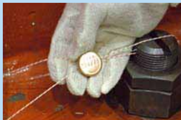
CAPS or commonly called the Metallic Seal is extensively used for sealing material containers and IAEA safeguards equipment.
