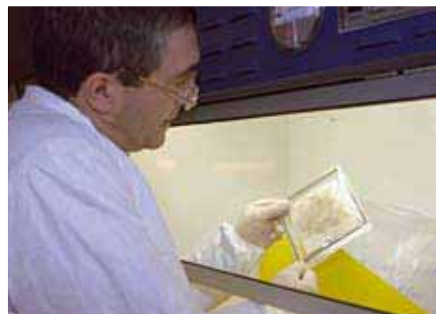
A technician prepares a swipe sample for screening at the SAL using X-ray fluorescence spectrometry.
