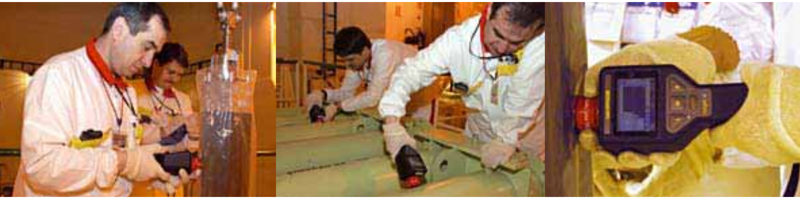
IAEA safeguards inspectors using the hand held HM-5 (fieldSPEC). The HM-5 is a modern hand-held digital gamma spectrometer combining various functions such as radiation dose rate measurement, nuclear material identification and isotope identification (e.g. U-235)
