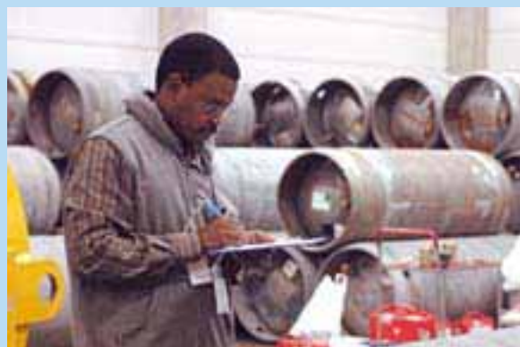
An inspector performing item counting of cylinders containing uranium hexafluoride (UF 6 ) used for uranium fuel fabrication.
