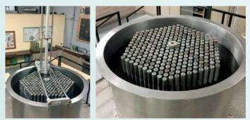
Nuclear detector handling system over the Nuclear-Chicago Modelo 9000 subcritical assembly
