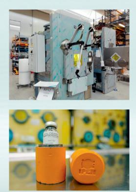
Hot cells (top) to prepare radiopharmaceuticals (bottom) after irradiation of various target materials at the Peruvian research reactor (IPEN)
