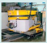
High resolution neutron diffractometer
