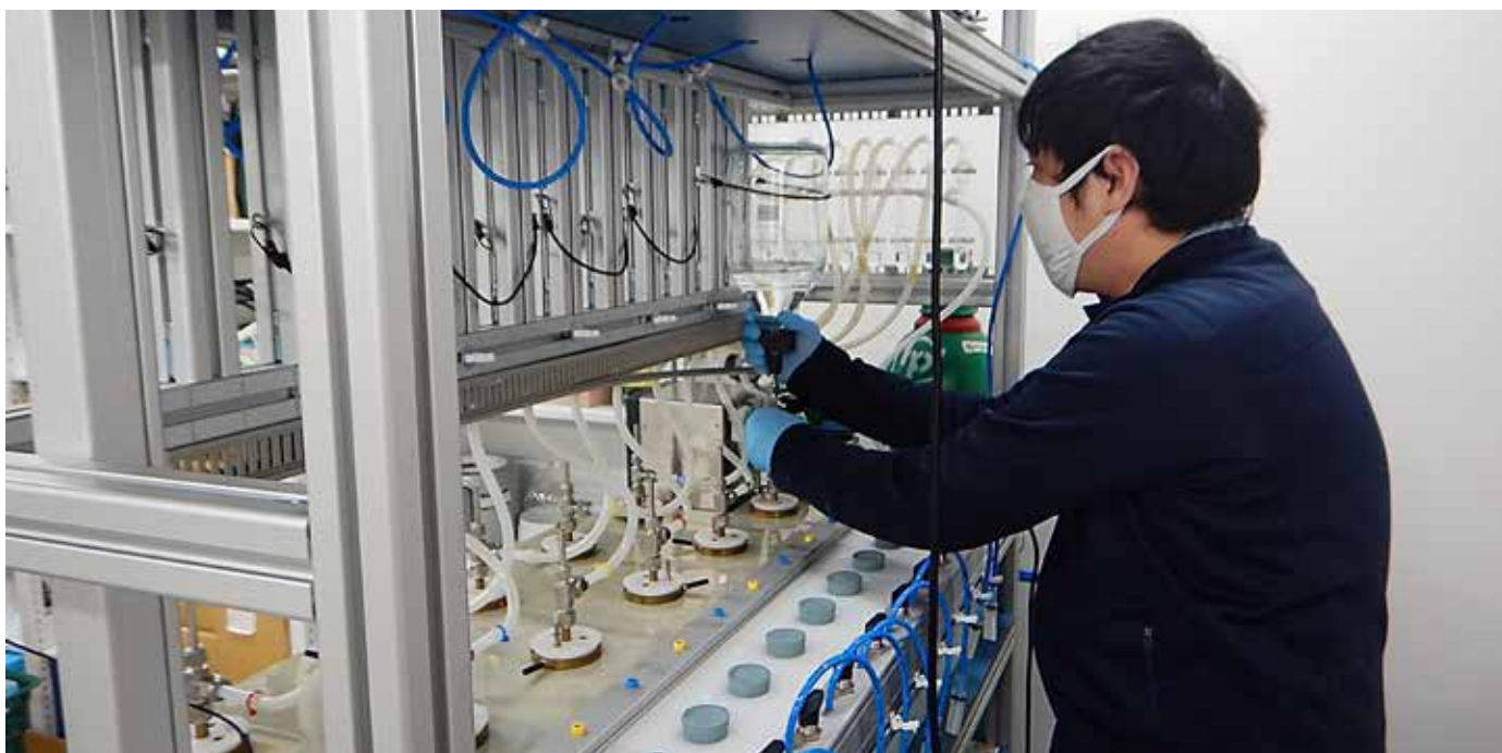
FIG. 9. Technical staff from Fukushima Prefecture working on the tritium enrichment system. (Photograph courtesy of the Fukushima Prefectural Centre for Environmental Creation.)
