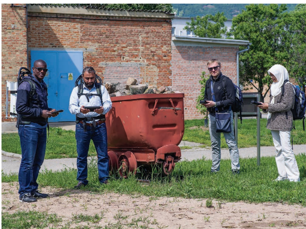
FIG. 3. Trainees equipped with gamma spectrometers and navigation systems undertake field measurements at a former uranium mine in Pécs, Hungary.
