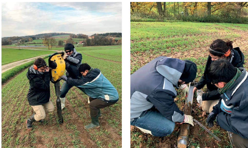
FIG. 3. Testing of a new radioisotope tracer to assess soil erosion as part of climate-smart agriculture.
