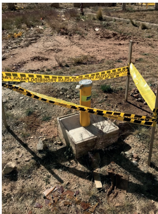
FIG. 1. One of several geological drills constructed as part of the site characterization for the new 200 kW research reactor in El Alto, Plurinational State of Bolivia.
