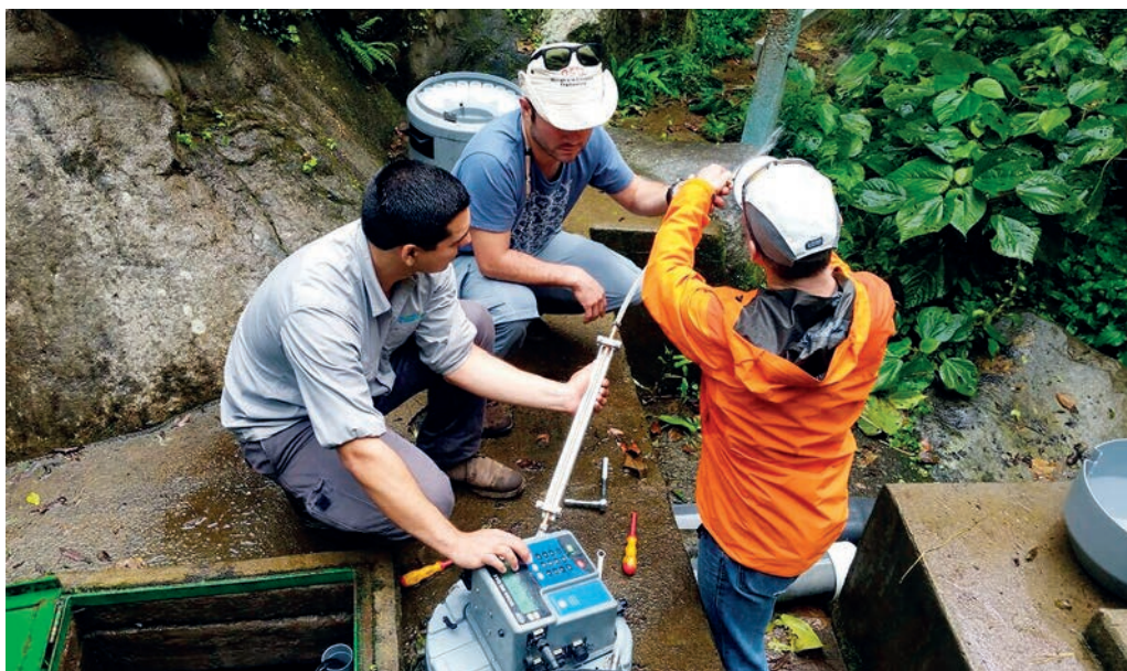
FIG. 1. Field training using groundwater sampling for analysis of noble gas isotopes in Costa Rica.
