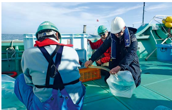
FIG. 3. Seawater samples from five stations within a 10 km radius of the Fukushima Daiichi nuclear power plant have been collected regularly since 2014 for interlaboratory comparisons between Japanese laboratories and the IAEA Environment Laboratories in Monaco. In 2016, interlaboratory comparisons were also organized for radionuclides in sediment and fish collected from the same area.
