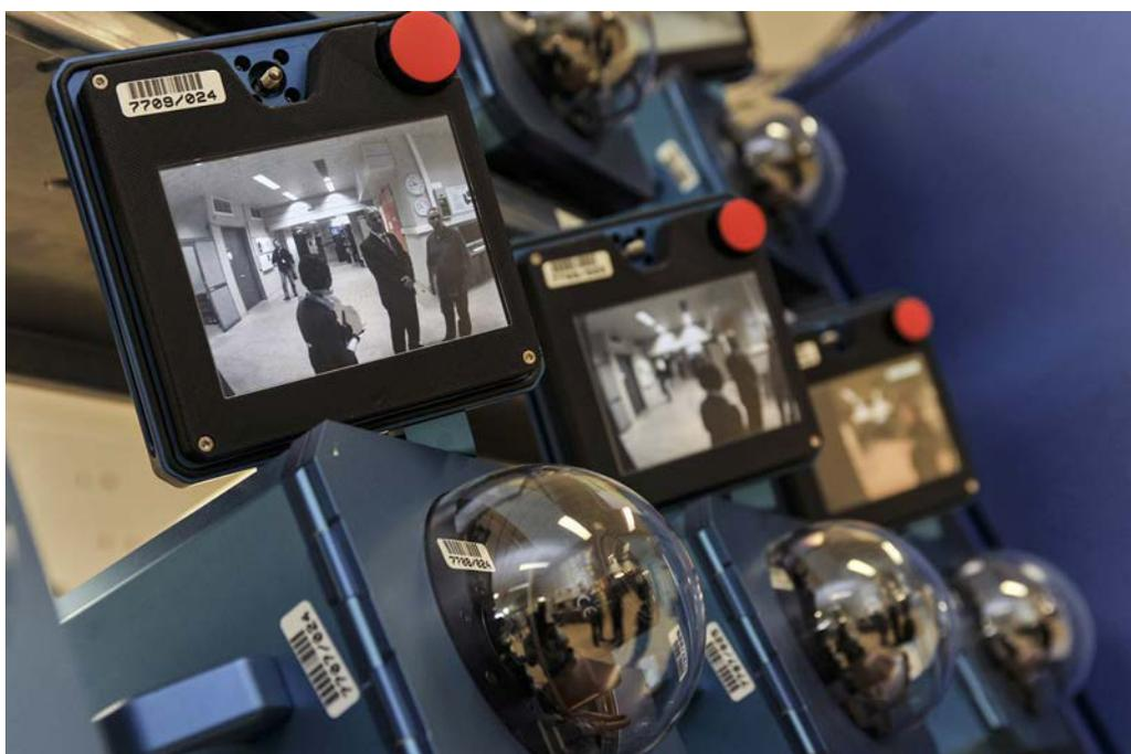
FIG. 2. Next generation surveillance system (NGSS) cameras undergo testing prior to installation in nuclear facilities.
