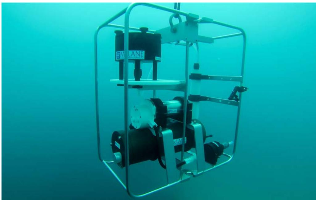
FIG. 1. Deployment of an underwater in situ pump for the collection and preconcentration of petroleum hydrocarbons for oil spill identification.
