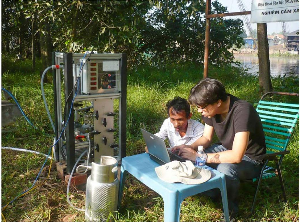
FIG. 1. Sampling for krypton-81 and noble gases for age dating of deep groundwater in the Mekong Delta Aquifer in southern Viet Nam.
