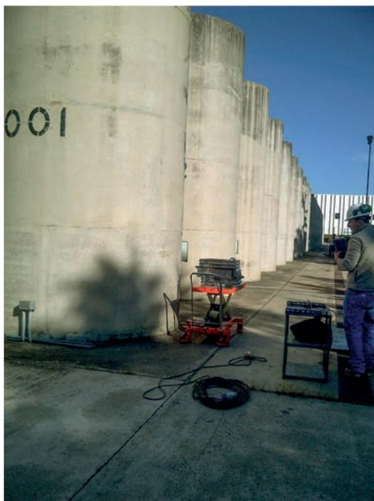
FIG. 2. Experts check the confinement integrity of the spent fuel and the structural integrity of the reinforced concrete silos at the Embalse nuclear power plant's dry storage, in Argentina, one example of research on the very long term storage performance of spent nuclear fuel and related storage system components supported through Agency CRPs. (Photograph courtesy of CNEA/NASA.)
