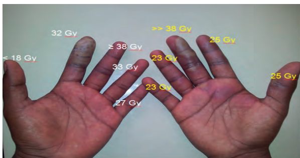
FIG. 3. Dose measured by electron paramagnetic resonance spectroscopy on fingernails of workers involved in an accident in Peru. (Photograph courtesy of IRSN, France.)
