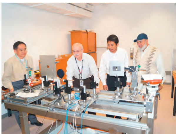
FIG. 2. Comparison measurements of national dosimetry standards in X ray beams during a technical meeting at the Agency's Dosimetry Laboratory in Seibersdorf.
