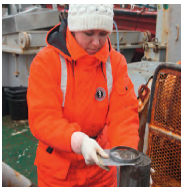
FIG. 2. Cutting a sediment core collected in the Kara Sea into vertical layers in order to investigate the historical contamination of radionuclides near dumped nuclear waste.
