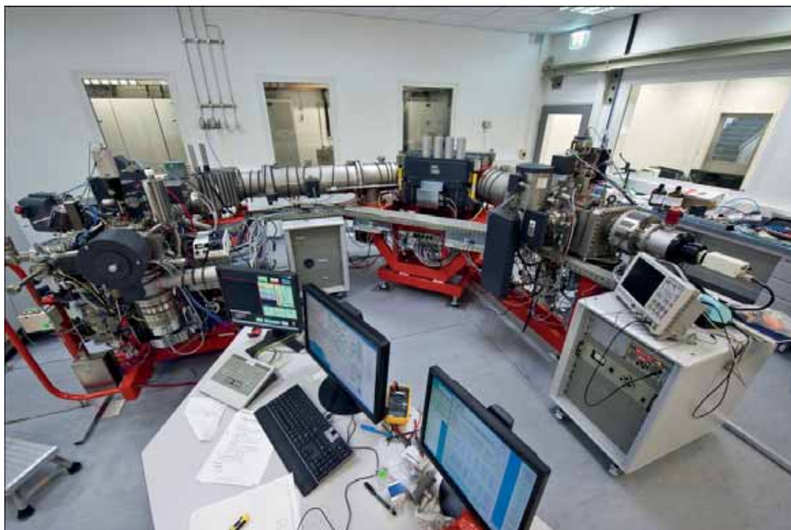
FIG. 3. CAMECA IMS 1280-HR Large Geometry Secondary Ion Mass Spectrometer in service in the Clean Laboratory extension, Seibersdorf.
