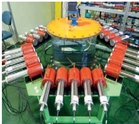
FIG. 3. Industrial single photon emission computed tomography system for the radiotracer visualization of ^{68}\text{Ga} and ^{137\text{m}}\text{Ba} from generators.
