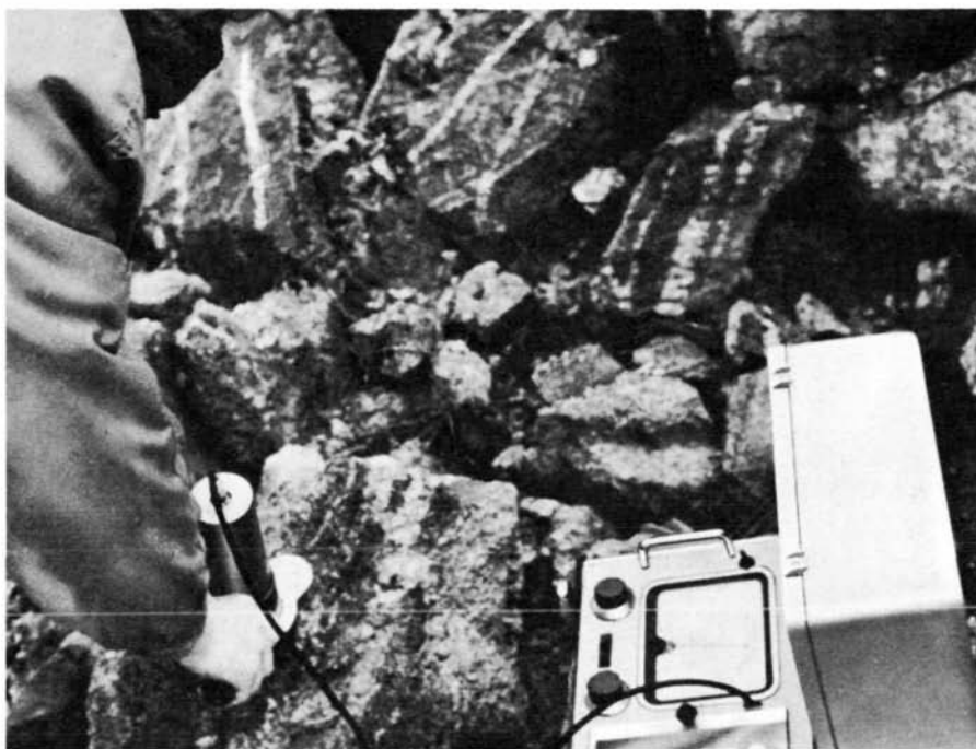
Prospecting for Tin Ore with the Isotope Portable Analyser (Photo: Hilger and Watts, Ltd.)
