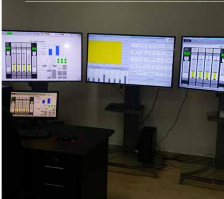
To support the training of JRTR operators and nuclear technology engineers, the JRTR training centre is equipped with a fully functional simulator. These simulators help them to understand and practice the ins and outs of research reactor operation, including possible safety incidents, so that they are well prepared to operate the reactor.
