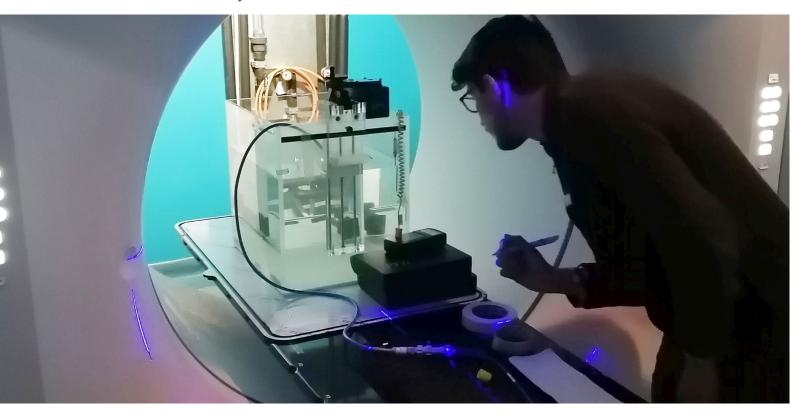
Specialist preparing a dosimetry setup for ensuring radiation doses are safe and accurate. (Photo: Tygerberg Hospital) Advances in radiotherapy technology are making cancer treatment more powerful, more precise and easier to deliver. While this means new benefits for patients, it also opens the door to new safety challenges.
