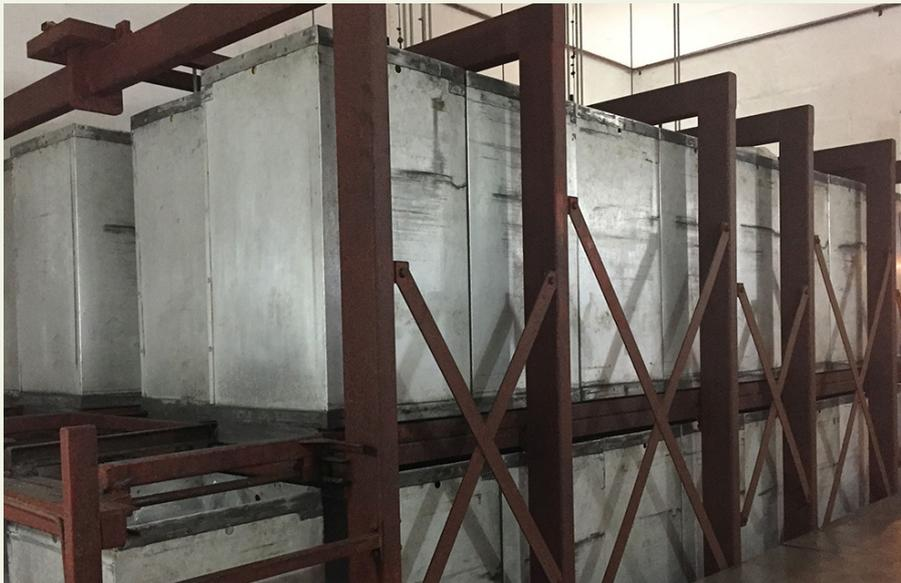
Food products undergo irradiation processes at VINAGAMMA using an electron beam irradiator, pictured here, and a gamma irradiator.
