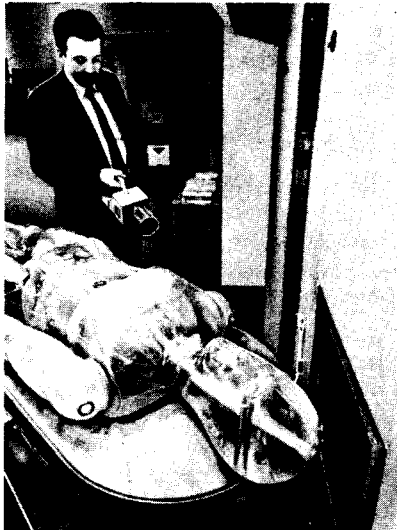
A "phantom" representing the human body at Brookhaven Laboratory. It is used to determine the rate at which neutrons travel in various parts of the body. The head, placed near the port of a medical research reactor receives the neutrons. (Phot. United Nations)
