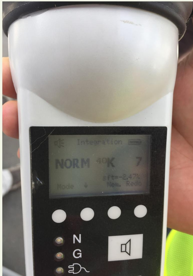
**A customs officer performing a secondary inspection on a truck that set off the port's radiation alarm. The handheld device confirms that the alarm was triggered by harmless amounts of naturally occurring radiation from potassium-40 isotopes, rather than from smuggled radioactive sources or nuclear material.**
