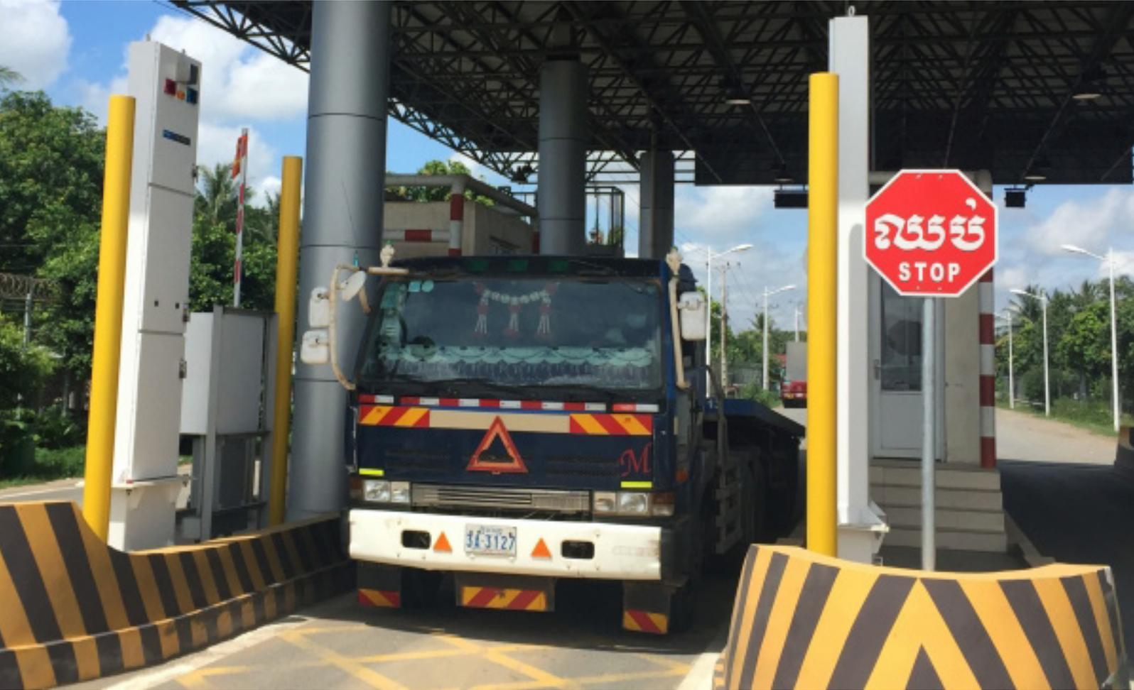
Every truck entering or leaving Cambodian ports passes through a radiation portal monitor – see the white panels with the red, orange and blue buttons. One third of shipments at the Phnom Penh port set off this alarm, even if they contain only harmless amounts of naturally occurring radiation. A new app developed by the IAEA will help customs officers zoom in on the shipments that may really contain smuggled radioactive material.
