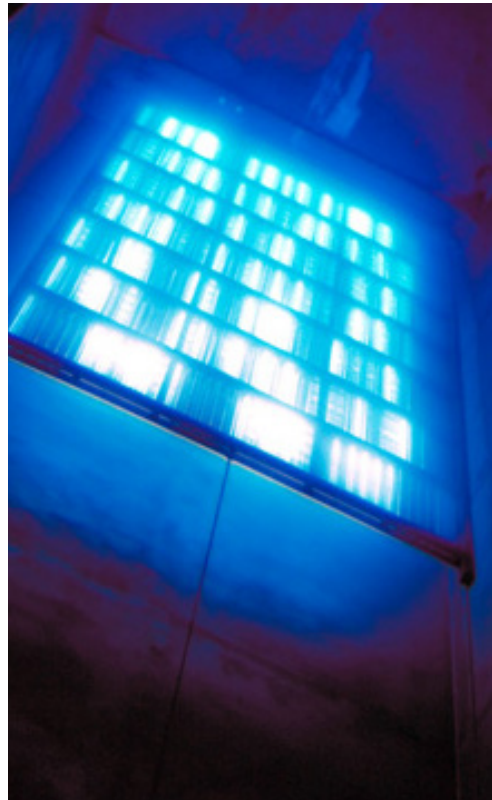
Cobalt-60 gamma irradiators are used to treat and sterilize materials for use in products such as packaging.
