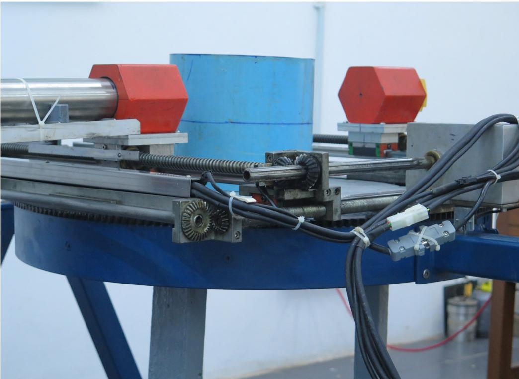
This NDT device emits radiation from the radioactive source (left). The radioactive particles react with the substance in the light blue pipe in the middle. The detector on the other side of the pipe measures radiation. This measurement provides information about the quality and quantity of the material going through the pipe.
