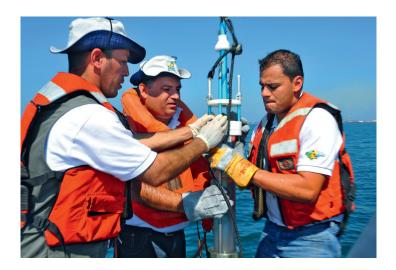
A team of scientists lowering core sediment sampling equipment off the coast of Honduras in 2009 to study the impact of water pollution using nuclear techniques. Photo: IAEA
