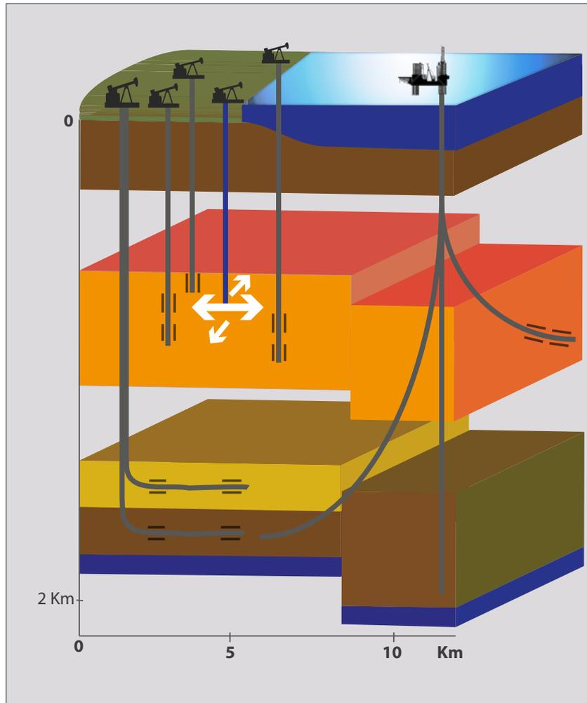
**Principle of tracer injection method for interwell communications**
