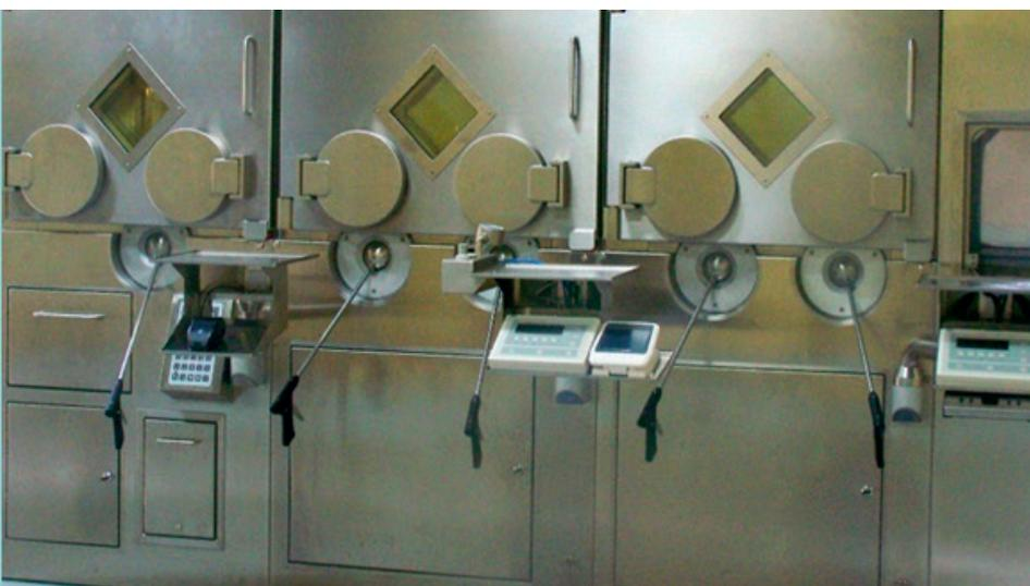
**The newly established facility for producing Y-90-based radiopharmaceuticals has good manufacturing practices compliant hot cells for protecting workers and ensuring the production of high-quality drugs.**
