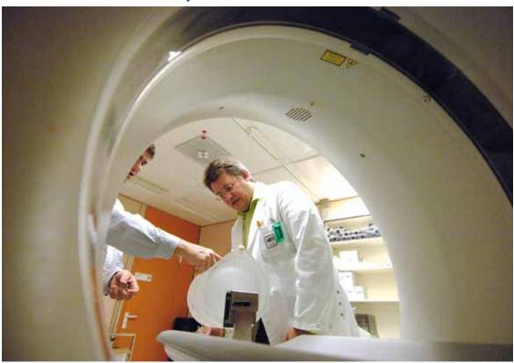
A physicist prepares a head phantom, which is a model of a head, for output measurements from a diagnostic imaging machine. (Photo: D. Calma/IAEA)
