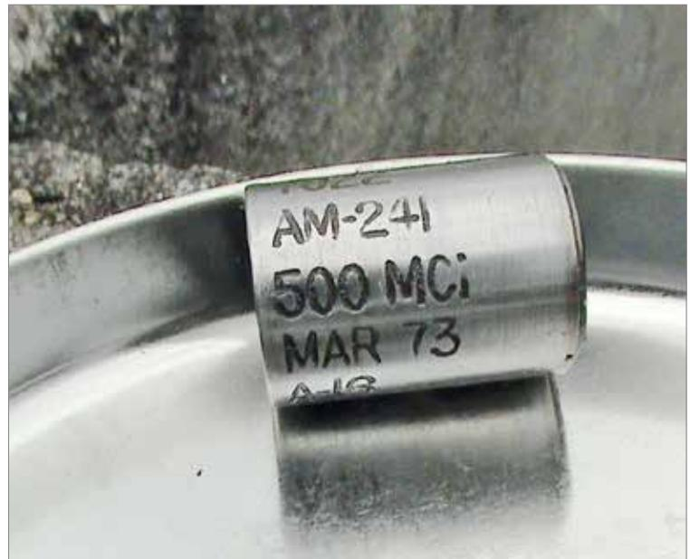
**4** Sealed radioactive sources or “sealed sources” are radioactive materials that have been isolated/sealed in metal capsules like this one. Sealed sources are used in many fields, such as medical diagnostics and treatment, to control industrial processes, and to sterilize food and medical products.
