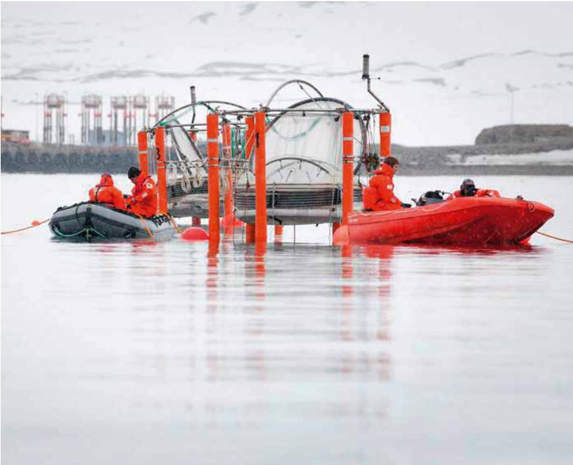
Radiotracer studies can be applied in floating or seabed tent structures called mesocosms. This valuable experimental tool allows natural environments to be studied under controlled conditions combining the benefits of lab and field work.
