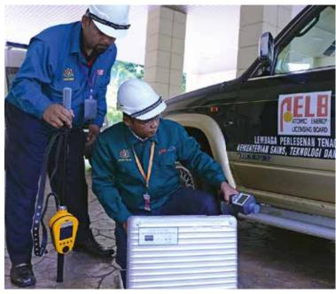
An AELB officer checks the radiation detection equipment before departing to inspect suspicious material.
