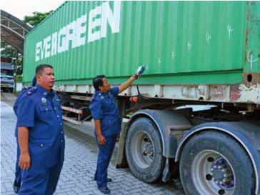
If customs officers determine the contents to be suspicious, they conduct a detailed radiation assessment using handheld radiation detectors. This equipment enables them to determine the exact radionuclide and the location of the material.
