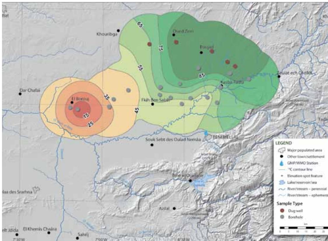
The plate from the *Hydrological Atlas of Morocco* showing water that is only minimally recharged as red areas. The green areas indicate water that is recharged.
