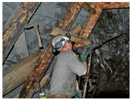
Miners drilling shot holes so they can blast out the uranium-bearing rock at Rozna I, the last active uranium mine in central Europe. They work up to 1200 metres below the surface, for six straight hours, five days a week. Because miners are exposed to ionizing radiation, they are only allowed to work 2100 shifts underground in their lifetime. For a number of years the Czech Republic has been between the eighth and the tenth largest uranium producer in the world.
