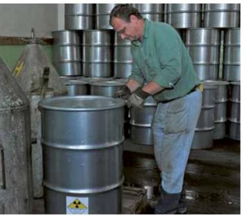
Yellowcake is packed in special, tightly sealed steel drums similar in size to oil barrels. Each weighs no more than 350 kg when full.
