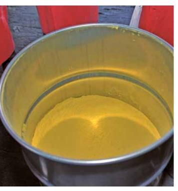
5 Uranium ore is processed into a concentrate known as yellowcake, which is produced at a plant a few kilometres from the mine.
