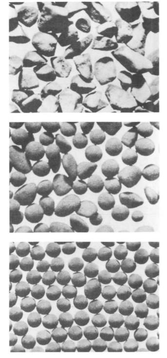
These three photographs, taken from the paper by H. Lloyd, show the progressive rounding of uranium diaxide granules by gyration. The picture on top shows the granules before being subjected to the gyration process, the one in the middle was taken after four hours' gyration and the one at bottom after nine hours' gyration
