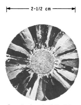
Cross-section of a uranium dioxide cylinder. (Picture reproduced from paper by G.E.Benedict and others)
