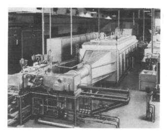
General view of a furnace for industrial sintering of uranium oxide. (Picture reproduced from paper by R. Hauser and A. Porneuf)
