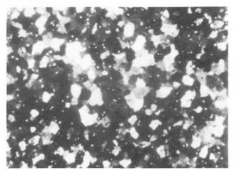
The microstructure of a hot-compressed solid solution of zirconium carbide and uranium carbide. (Picture reproduced from a paper by R.B. Kotelneekov and others)
