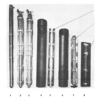
Some of the magnox fuel elements manufactured by the UK Atomic Energy Authority. 1. Calder Hall element; 2. Latina element; 3. Bradwell Mk III element; 4. Tokai-Mura graphite sleeve; 5. Tokai-Mura element; 6. Hunterston sleeve; 7. Hunterston element; 8. Berkeley Mk. 1B. (Picture reproduced from paper by C. Allday)
